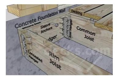
When attaching to solid masonry, you will have to install expansion anchors with a minimum diameter of 1/2" and set into the wall at least 2 1/2". Hollow concrete block can easily break when drilled and doesn't leave adequate bearing support for anchors. If you are attaching to a hollow masonry wall, you can fill the cells with grout and use expansion anchors, or you'll need to install epoxy anchors in compliance with the manufacturer's installation instructions to a minimum depth of 4 1/4".
